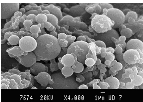
Figure 7 SEM micrographs of AZT-loaded PLGA microparticles.
